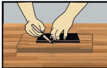
MARK AND CUT THE FLOORING MATERIAL
